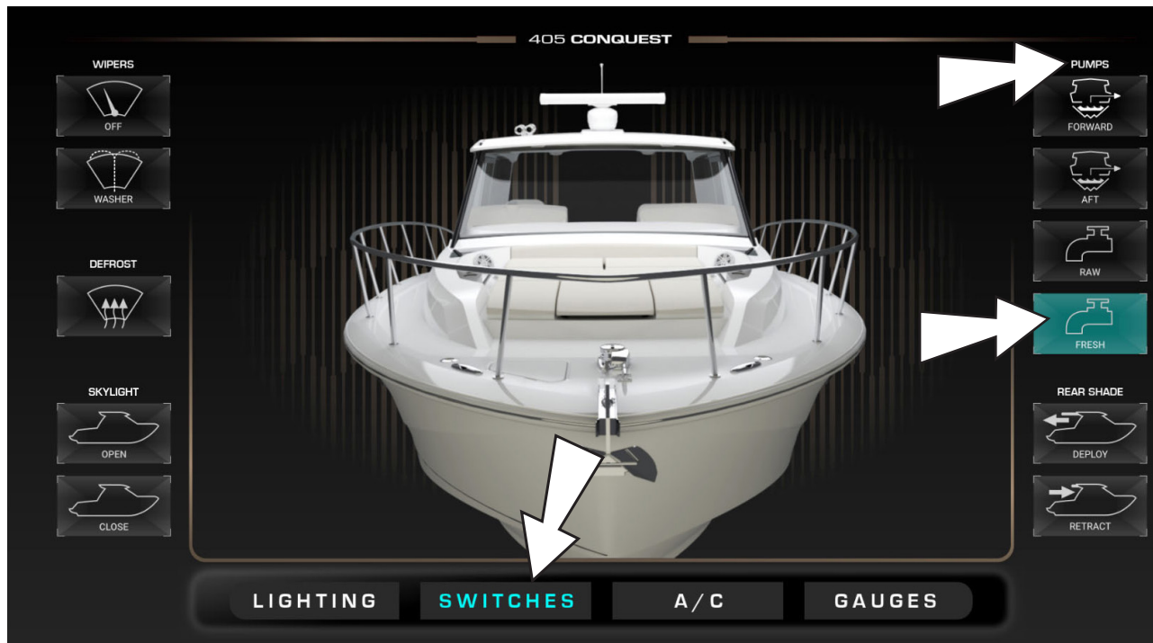
Switches Tab, Raw Water Figure 3.19.1
