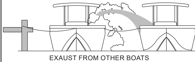
Examples of accumulation of Carbon Monoxide Fig. 1.7.1
