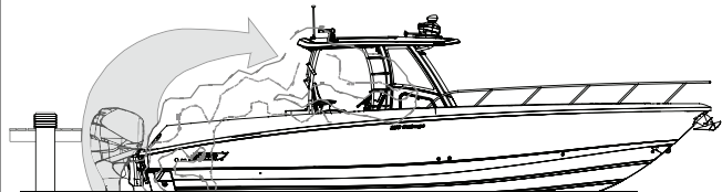
BLOCKAGE OF EXHAUST BY OBSTRUCTION
