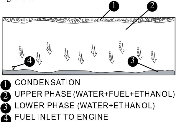
water and ethanol, is deep enough to reach the fuel inlet, it could be pumped directly to the engine(s) and cause significant problems. Engine problems can also result from the reduced ethanol/fuel mixture left in the upper phase of the tank.
