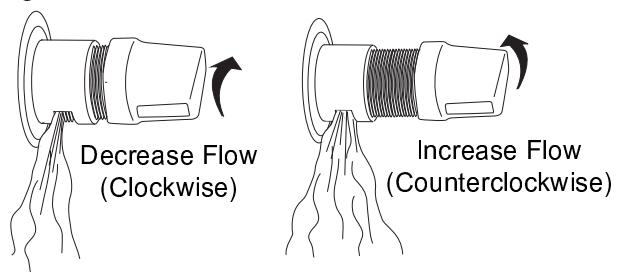
A flow control valve (Figure 3.8.2) at the livewell water inlet controls the flow of water into the livewell. To increase the water flow, turn the valve counterclockwise. To decrease flow, turn the valve clockwise.
