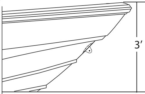
will make it easier to mount a trolling motor. The reinforced sections are located on either side of the bow navigation light and extend back along the gunwale. The phenolic material can be drilled and tapped to hold machine screws.
